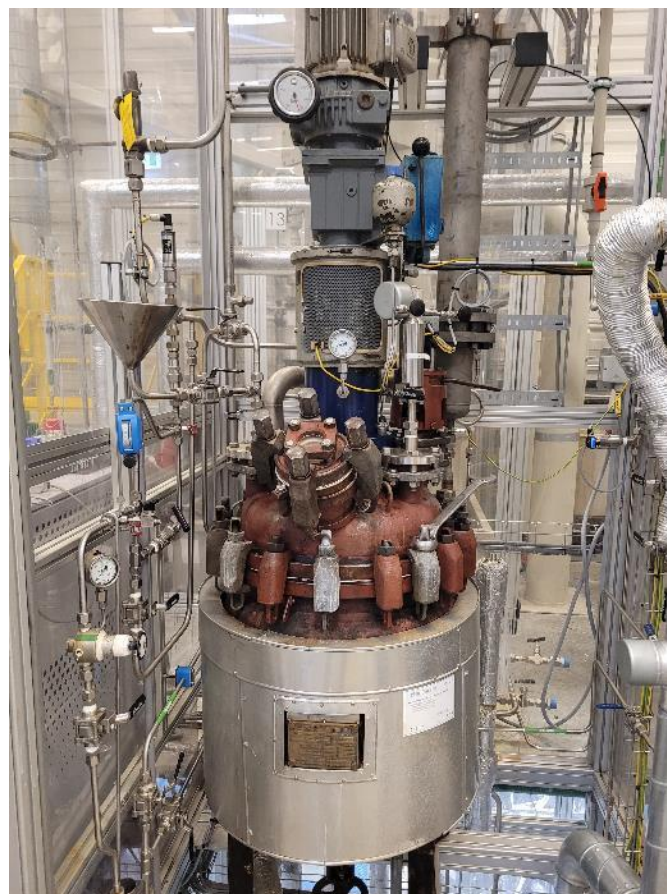
Pilot plant 20 l hydrogenation unit
